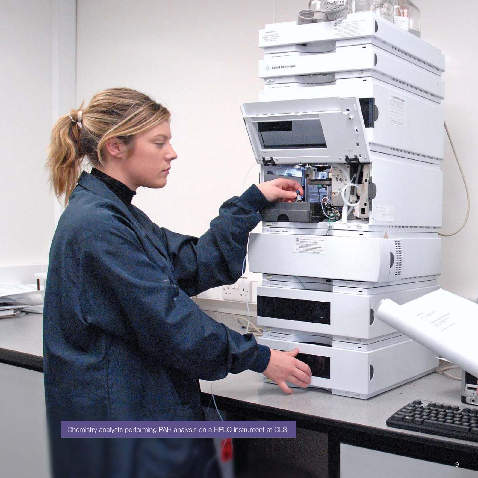
Chemistry analysts performing PAH analysis on a HPLC instrument at CLS
